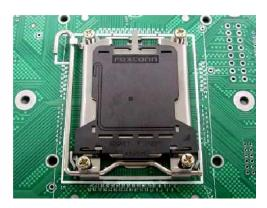
NOTE: Do not assemble CPU before securing socket with screws.
